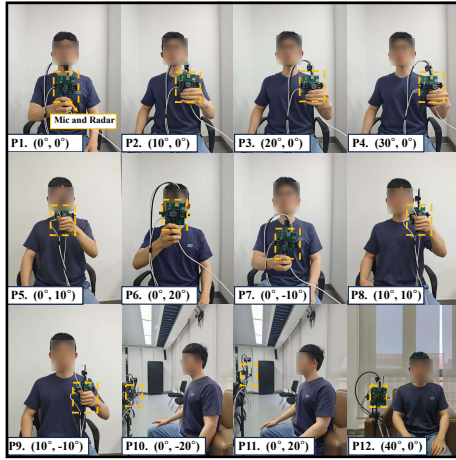
Fig. 29. Device placement configurations in real-world usage scenarios. The angles in parentheses indicate the horizontal and vertical AoA.
