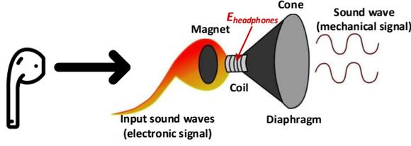
Figure 2: An illustration of headphones' working principle.
