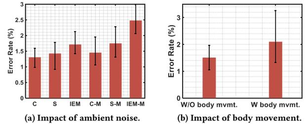
Figure 21: Error rate of the heartbeat rate estimation. (a) We measure the error rate both in the absence (the first three columns) and in the presence (the last three columns) of the audio input signal. (b) We measure the error rate both in the absence and presence of strong body movements.
