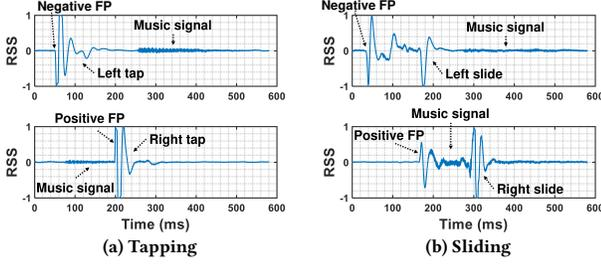
Figure 22: The voltage output signals  $V_g$  caused by different touch-based gestures. (a) tapping the left (top) and right (bottom) enclosure. (b) sliding on the left (top) and right (bottom) enclosure.
