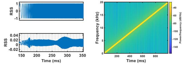
**Figure 14: An illustration of chirp signal. (a) The transmitted (top) and received chirp signal in time domain. (b) The spectrogram of a transmitted chirp whose frequency spans from 20 Hz to 20 kHz in one second.**
