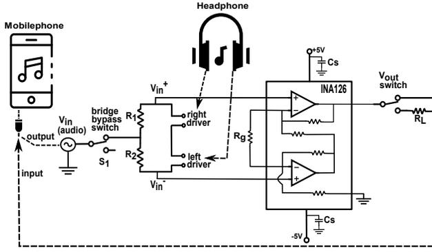
Figure 8: Schematic of HeadFi.
