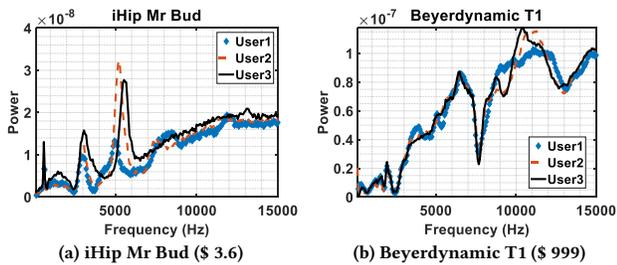
Figure 15: Channel response of three persons characterized by (a) low-end and (b) high-end headphones.
