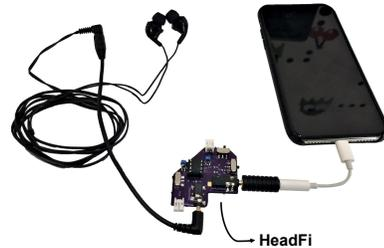
**Figure 1: Illustration of HeadFi prototype.** HeadFi works as a plug-in peripheral that connects a pair of headphones and a smartphone. It captures the minute voltage change on the headphones’ drivers and offloads voltage readings to the smartphone for processing. HeadFi can be miniaturized and further embedded into a smartphone as an integrated circuit.
