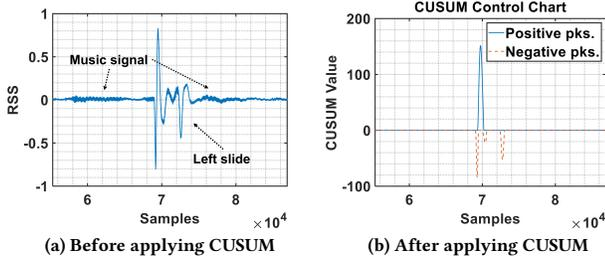
Figure 23: Output signal  $V_g$  before and after applying CUSUM.
