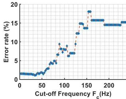
Figure 20: The heartbeat monitoring error rate is low when  $F_c$  is below 50 Hz.
