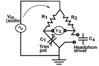
Figure 7: Null measurement in the Wheatstone bridge.
