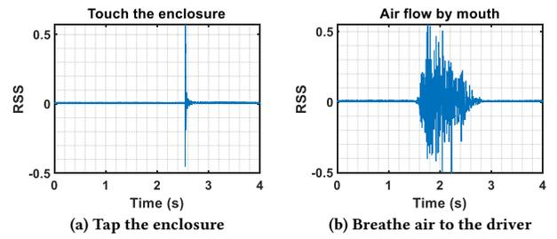
**Figure 13: Time domain signal when the headphones are placed on a table. (a) The enclosure is tapped by a finger and (b) breathing air to the driver.**
