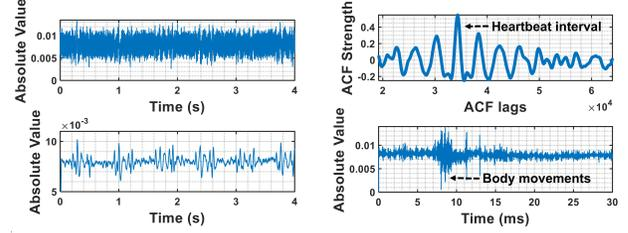
**(a) The voltage output before and after filtering. (b) The ACF plot and time domain interference.**
