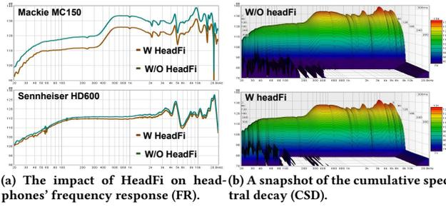
**Figure 12: The impact of HeadFi on headphones. (a) The FR of a high-quality (Sennheiser HD600, \$399.95) and low-quality (Mackie MC150, \$49.0) headphones in the presence and absence of HeadFi, respectively. (b) A CSD snapshot of Mackie MC150.**
